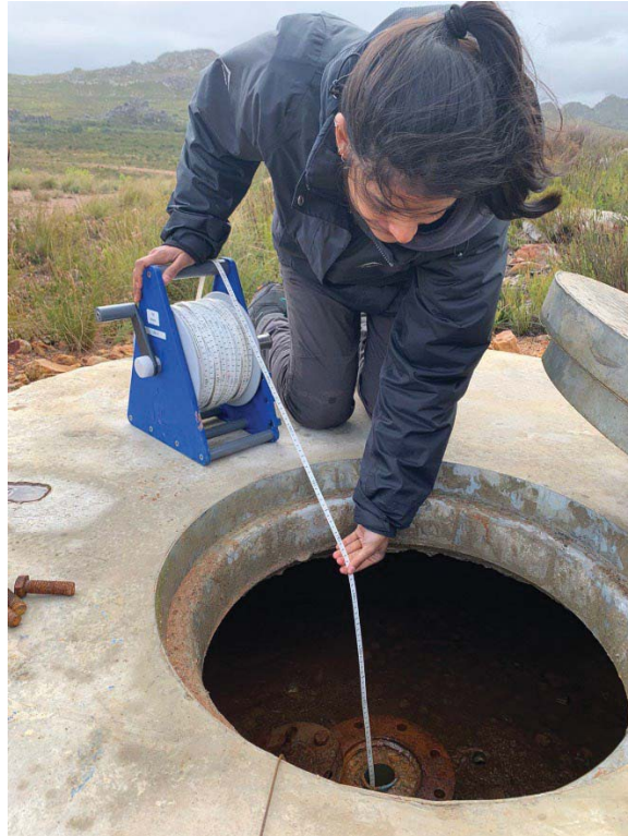
Figure 2-8 Dip meter used to measure groundwater levels.
